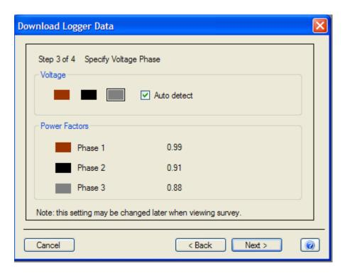
This screen shows the results of the autodetect sequence for voltage phase detection. In this example ph3 has been selected, and the resulting phase power factors shown in the lower pane.
