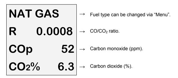
Press to print a full combustion test, (or send to PC via optional Wireless module).
