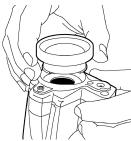
5. Carefully push the lens into position.
