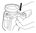
2. Rotate the lens counter-clockwise 30° (looking at the front of the lens).
