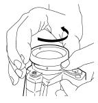
3. Carefully pull out the lens from the bayonet ring.
