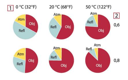
**Figure 35.2** Relative magnitudes of radiation sources under varying measurement conditions (SW camera). 1: Object temperature; 2: Emittance; Obj: Object radiation; Refl: Reflected radiation; Atm: atmosphere radiation. Fixed parameters:  $\tau = 0.88$ ;  $T_{refl} = 20^{\circ}C$  (+68°F);  $T_{atm} = 20^{\circ}C$  (+68°F).
