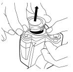
4. Correctly position the lens in front of the bayonet ring.
