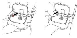
4. Pull out the battery from the battery compartment.
