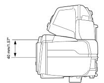
Figure 8.1 This figure shows the difference in position between the laser pointer and the optical center of the infrared lens.
