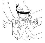
3. Carefully pull out the lens cap from the bayonet ring.
