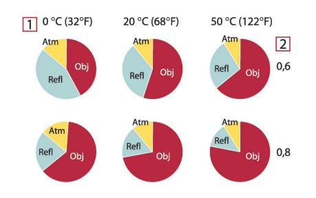
**Figure 35.3** Relative magnitudes of radiation sources under varying measurement conditions (LW camera). 1: Object temperature; 2: Emittance; Obj: Object radiation; Refl: Reflected radiation; Atm: atmosphere radiation. Fixed parameters:  $\tau = 0.88$ ; T<sub>refl</sub> = 20°C (+68°F); T<sub>atm</sub> = 20°C (+68°F).
