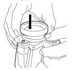
6. Rotate the lens 30° clockwise (looking at the front of the lens).
