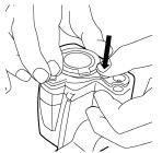
2. Rotate the lens cap 30° counter-clockwise (looking at the front of the lens).
