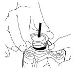
6. Rotate the lens cap 30° clockwise (looking at the front of the lens).
