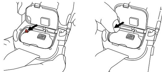
4. Pull out the battery from the battery compartment.
