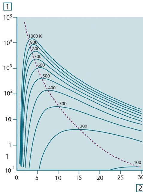
**Figure 34.6** Planckian curves plotted on semi-log scales from 100 K to 1000 K. The dotted line represents the locus of maximum radiant emittance at each temperature as described by Wien's displacement law. 1: Spectral radiant emittance ( $\text{W}/\text{cm}^2$  ( $\mu\text{m}$ )); 2: Wavelength ( $\mu\text{m}$ ).
