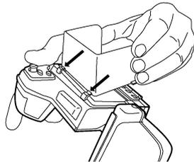
3. Carefully hold together the two rear wings of the sunshield.
