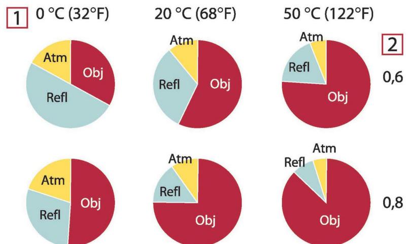
**Figure 35.2** Relative magnitudes of radiation sources under varying measurement conditions (SW camera). 1: Object temperature; 2: Emittance; Obj: Object radiation; Refl: Reflected radiation; Atm: atmosphere radiation. Fixed parameters:  $\tau = 0.88$ ;  $T_{\text{refl}} = 20^{\circ}\text{C}$  ( $+68^{\circ}\text{F}$ );  $T_{\text{atm}} = 20^{\circ}\text{C}$  ( $+68^{\circ}\text{F}$ ).
