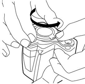
3. Carefully pull out the lens cap from the bayonet ring.
