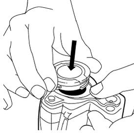
6. Rotate the lens cap 30° clockwise (looking at the front of the lens).
