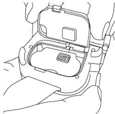
3. Push the red release button in the direction of the arrow to unlock the battery.
