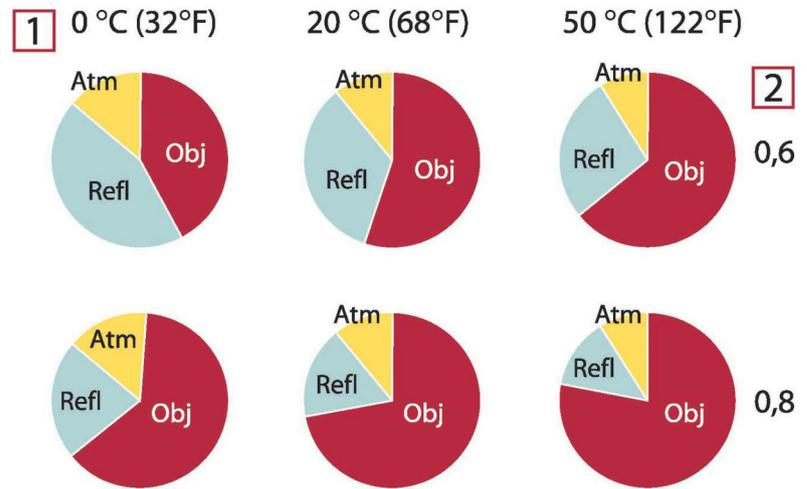
**Figure 35.3** Relative magnitudes of radiation sources under varying measurement conditions (LW camera). 1: Object temperature; 2: Emittance; Obj: Object radiation; Refl: Reflected radiation; Atm: atmosphere radiation. Fixed parameters:  $\tau = 0.88$ ;  $T_{\text{refl}} = 20^\circ\text{C}$  (+68°F);  $T_{\text{atm}} = 20^\circ\text{C}$  (+68°F).
