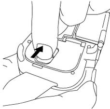
2. Open the cover to the battery compartment.
