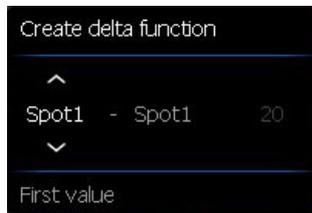
3. Push the joystick. The result of the difference calculation is now displayed on the screen.
