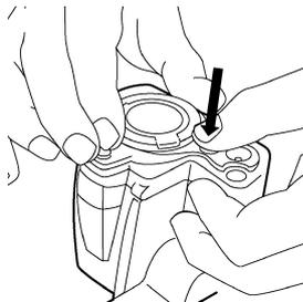
2. Rotate the lens cap 30° counter-clockwise (looking at the front of the lens).
