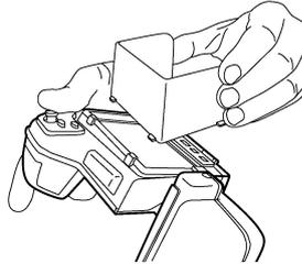
2. Push the front part of the sunshield into position. Make sure that the two tabs mate with the corresponding notches.
