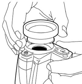
5. Carefully push the lens into position.
