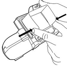
4. Push the rear part of the sunshield toward the screen, and then release your grip. Make sure that the two tabs mate with the corresponding notches.
