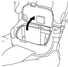
3. Push the battery into the battery compartment until the battery-locking mechanism engages.
