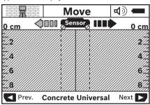
Position the measuring tool against the wall and move it over the wall in the direction of travel (see "Method of Operation", page 16). Measured results are indicated on display 16 after a minimum measuring distance of 10 cm. To ensure correct measurement results, move the measuring tool slowly and completely over the assumed object in the wall.
