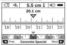
In the example, rule mode shows the same situation as in figure D: Three steel bars equally apart. In rule mode, the clearance between the detected object centres can be determined.
