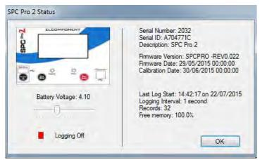
Battery voltage should read over 3.7 volts. If it is lower than this the logger may shutdown if it is not connected to a mains supply.
