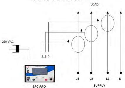
**NOTE**: It is <u>essential</u> to orientate the CTs with the arrow pointing <u>towards the load</u> as shown.
