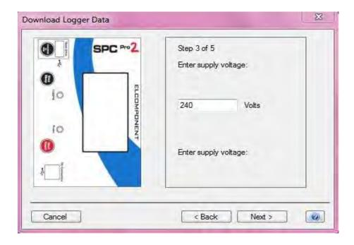
This screen appears if the software detects that no voltage was measured consistently through the survey (e.g. battery powered survey), and manual input is required.
