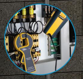
Inductive clamp allows you to induce a tracer signal on to the cable without affecting the low voltage signals on the circuit. Individual wires can be sorted, opens can be located and shorts can be isolated.
