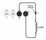
**B]** Current generated by external source (ammeter panel input used).
