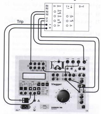
Connect for testing as shown in the above diagram.
