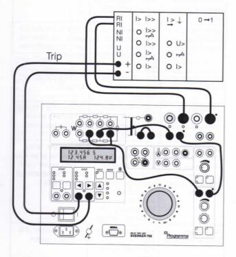
The SVERKER voltage source can supply the output transformer via a reverse circuit comprising two parallel-coupled resistors of 1000  $\Omega$  and 500  $\Omega$ . See illustration above.
