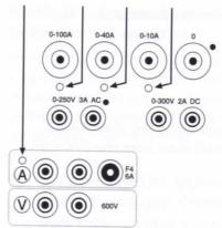
Use the button marked A to transfer the ammeter test point to the selected input.
