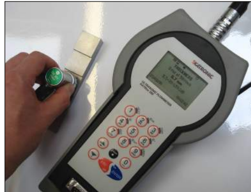
Wall thickness gauge used with KATflow 200
