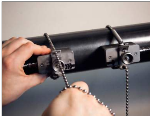
Transducers mounted using clips and chains
