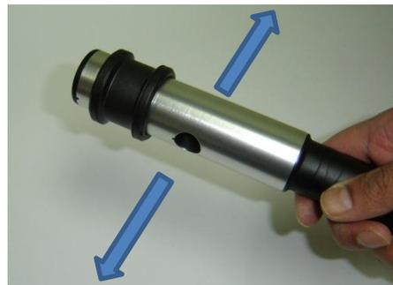
If sampling via a gravimetric adapter, especially at high concentrations, it is recommended to orientate the probe in a horizontal axis as shown. This enables dust to fall through the sampling chamber thus reducing the risk of optical contamination. If the probe is aligned vertically, there is an increased risk of particulate material 'settling out' due to gravity and subsequently dropping down inside the probe.
