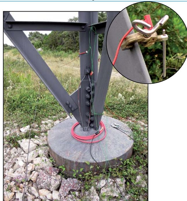
By using AmpFLEX™ sensors, you can measure on any pylon configuration.
