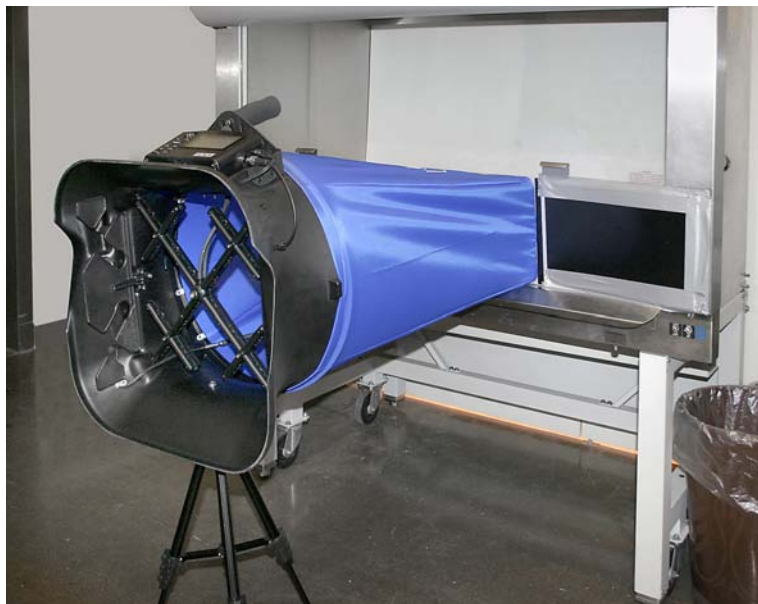
Figure 21: Direct Inflow Measurement Hood
