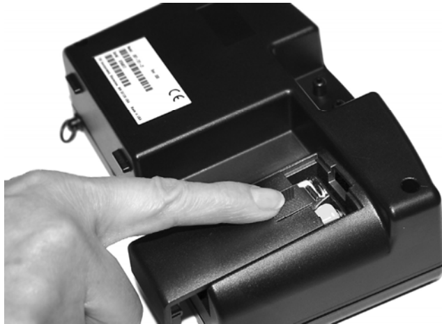
Figure 4: Battery Cover Removal
