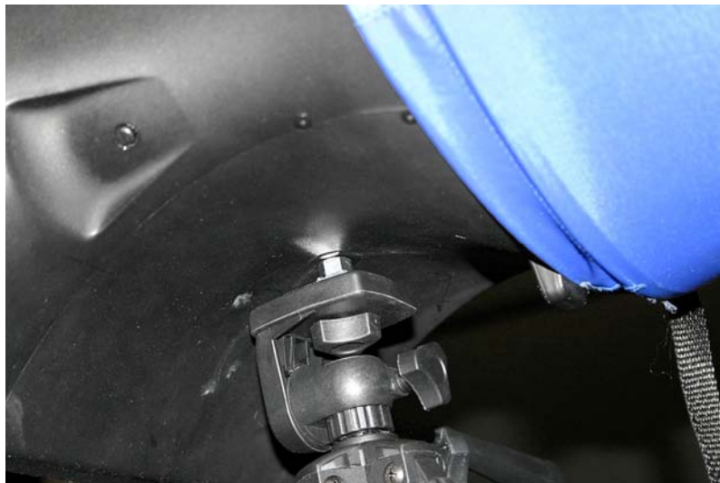
Figure 25: Mount Hood Base to Telescopic Stand
