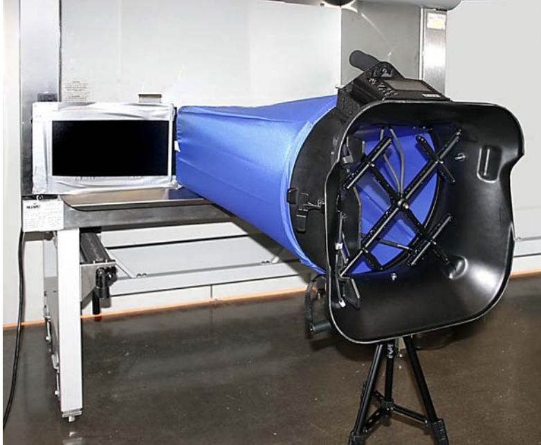
Figure 26: Adjust Height and Position of Telescopic Stand
